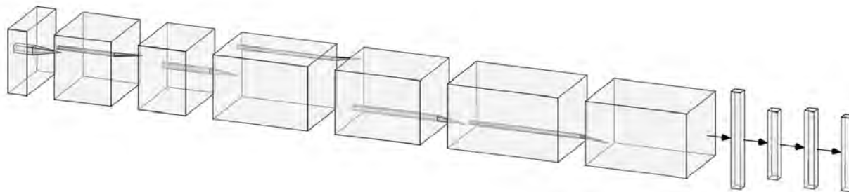
Figure 6: Convolutional Neural Network Model Architecture (image generated using [4]).
